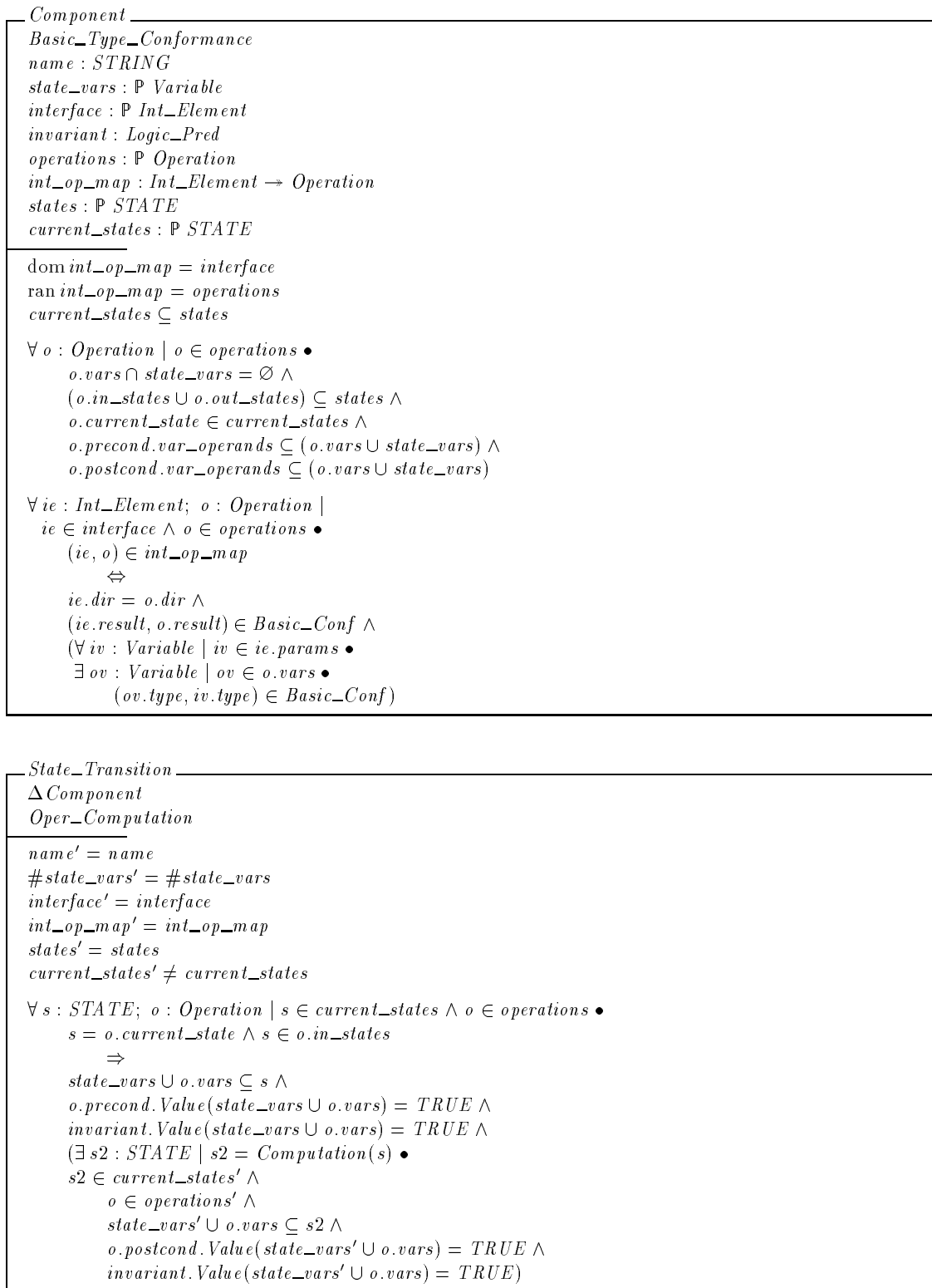
Figure 4-3. Z specification of architectural types (components).
