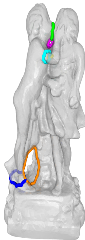
Figure 1. Fundamental cycles generated by our flexible control of cycle computation on a triangle mesh with 50,000 faces. The six cycles computed in this genus 3 model were found using a simple breadth-first construction of the spanning tree to guide our algorithm.
