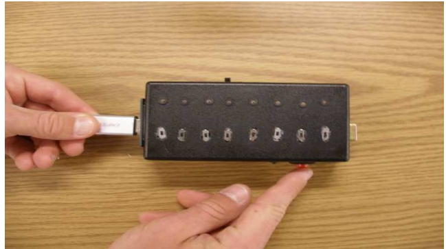
Figure 4: The virtual microcontroller is programmed by simply plugging in a USB flash drive with the V \mu C program and pressing a button.
