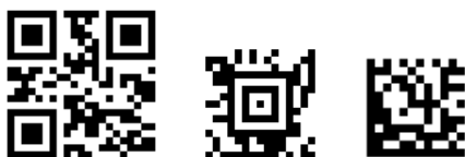
Figure 5. Popular 2D Barcodes with rectangular pixels: Quick Response, Aztec, Data Matrix
