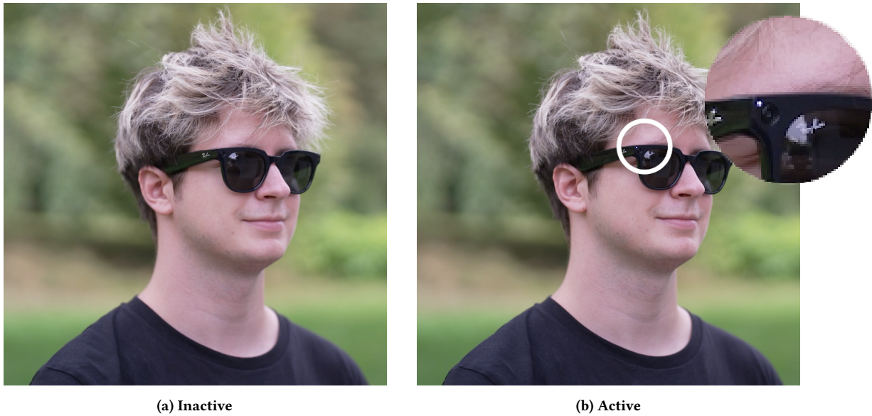
Figure 7: Depiction of the glasses before and during a recording. The active LED indicator is magnified.
