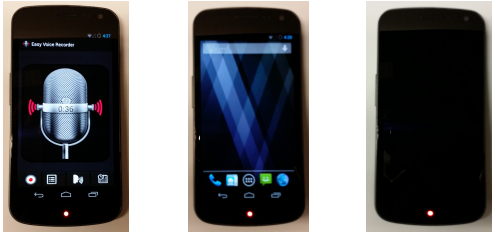
Figure 1: LED notification for microphone using Viola. The LED blinks even if the application is in the background or if the display is off. Malicious attempts to break this notification will be blocked.
