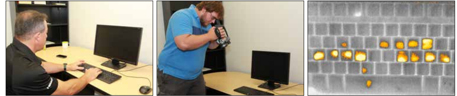
Up to one minute after a victim enters a password (left), someone with a thermal camera (center) can capture the keys pressed – in this case, “i love you” (right).
