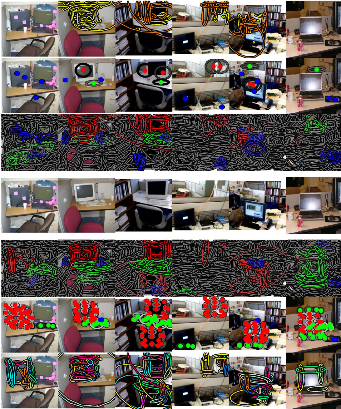
Figure 6.18. Additional feature segmentations produced by TDP models of office scenes containing computer screens (red), keyboards (green), mice (blue), and background clutter (gray). We compare a simplified TDP model which describes object shape via a single Gaussian cluster (top rows) to the full, multiple-part TDP model (bottom rows) of Fig. 6.12. Row 4: Six test images. Rows 3 & 5: Segmentations for each model, in which features are assigned to the object category with the highest posterior probability. Rows 2 & 6: Parts corresponding to the objects instantiated at a single Gibbs sampling iteration (background clutter not shown). Rows 1 & 7: Color-coded assignments of features to different parts and instances of the screen category.
