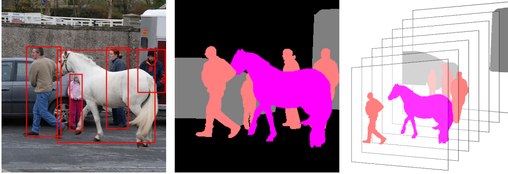
Figure 1. Our framework. Multi-class object detections algorithms typically predict bounding box locations and class labels ( left ). Such reports only provide relatively coarse reports about objects. Multi-class segmentation algorithms provide class labels for every pixel ( center ). We propose to use object-specific bounding box representations to guide multi-class segmentation algorithms. To do so, we introduce layered representations ( right ) that reason about relative depth orderings of objects. Layered representations are helpful, for example, to link object segments separated by an occluder (e.g., the center person occluded by the horse).
