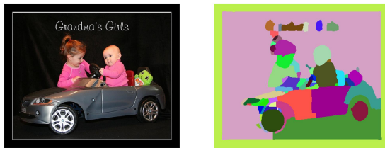
Figure 4. We show an example superpixel grouping from [1] tuned to return roughly 200 superpixels. We use this bottom up information in our probabilistic model by conditioning on the fact that all pixel labels from within a superpixel must share be identical.
