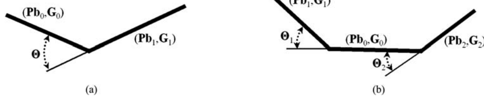
Fig. 10 (a) A simple 2-edge model of local curvilinear continuity. Each edge has associated features: the average Pb and whether it is a G -edge or C -edge. Continuity is measured by the angle \theta . The edge pair is either classified as a continuation ( X_{e_0} = 1, X_{e_1} = 1 ) or not.
