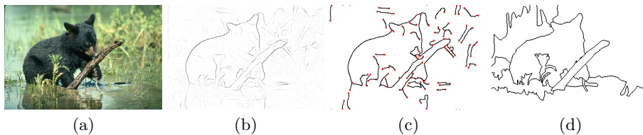
Fig. 8. Constructing contour/junction structure (c) from thresholded Pb edge maps (b). Contours are marked in black and junctions in red. Such a discrete structure allows global inference on junction consistencies. However, bottom-up contours are much more fragmented and not nearly as clean (and useful) as the human-marked boundaries (d).
