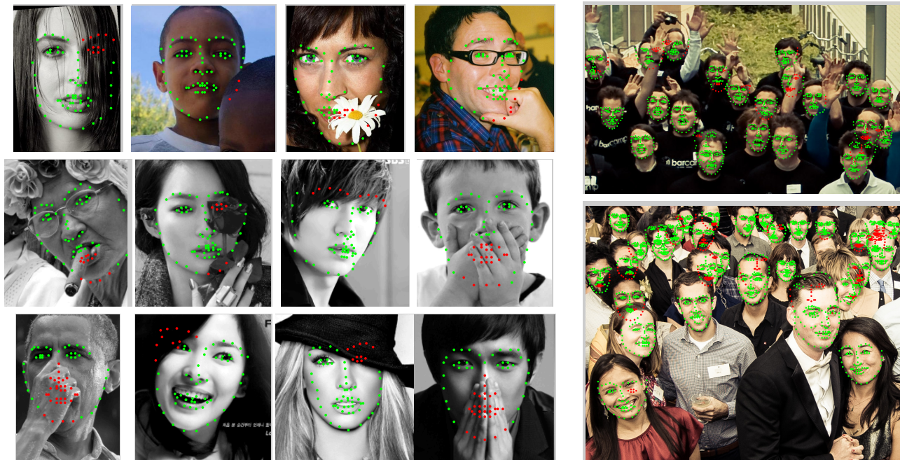
Figure 6. Right: Examples of landmark localization and occlusion estimation for images from the HELEN (row 1) and COFW (rows 2-3) test datasets. Left: Examples of detection and localization in scenes with substantial occlusion. Red indicates those keypoints which are predicted as being occluded by the HPM.
